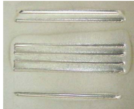
Nitinol coupon pattern etched and polished to an R_a < 120 \text{ nm} .
