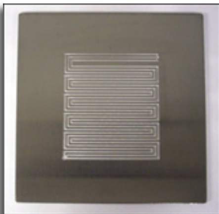
Sample 430 stainless steel bipolar plate with gas flow fields formed using The FARADAYIC ElectroEtching Process
